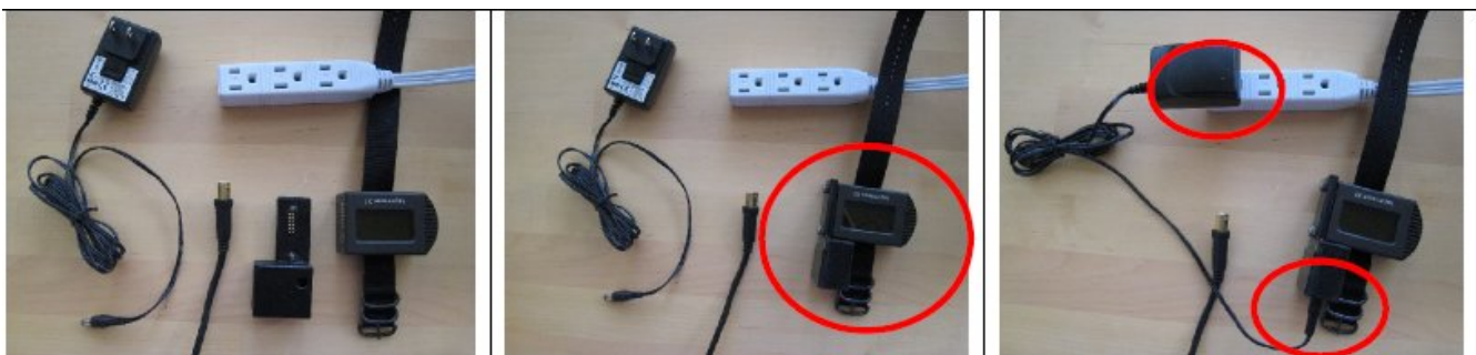
1. Prepare all the cables... 2. FIRST connect the attachment to the X1 using the thumbscrews... 3. THEN connect to the AC adapter and to the power supply...
